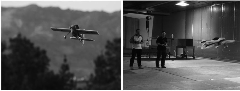
Fig. 1 Flight tests of the variable-configuration UAV in calm-wind open-air flight (configuration 2a, left) and in the turbulent wind tunnel (configuration 3a, right). See Table 1 for configuration details.
